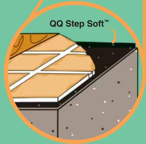
This high-frequency noise dampener works from 1000 hz and up to soften the impact noise of footfall in systems in which there is already ample airborne noise control, and no additional mass is required to achieve the Sound Transmission Classification ASTM standard required under the International Building Code.
