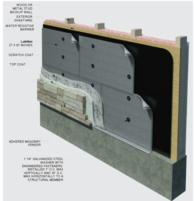
**Product:** Subject to compliance with requirements, provide "Driwall LathNet™" as manufactured by Mortar Net Solutions™.
