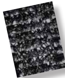
Drivall™ PCD is 0.125 - 0.75 inches thick (3.175 - 19.0 mm thick)
